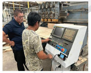
With compact design, DNC device doesn't take too much space. Furthermore DNC device also hve many useful features that will helps the operators saving time such as: Data transmit through Wi-fi, checking the shape of working program, toolpath, the operators also can edit program directly on DNC device without using computer. QS Technology Micro DNC device has been being widely used in many industry domains such as: Mold making, Wire CNC cutting, Machining (Milling / Turning), ....
