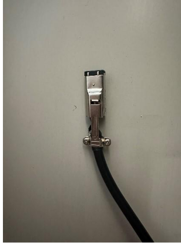
Figure 2-20. I/O link cable using shield wire and be soldered to the controller
