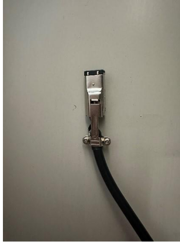
Figure 2-24. I/O link cable using shield wire and be soldered to the controller
